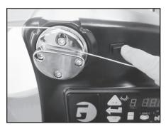
To tension a string, push the tension switch or the foot pedal. The string gripper will rotate and slowly apply tension to the string. When the set tension has been attained, the gripper will stop rotating and the display will flash. As the tensioned string stretches, the gripper may rotate intermittently, maintaining the set tension.
